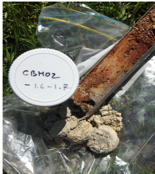
Photo 12: Sandstone encountered at CBH02
