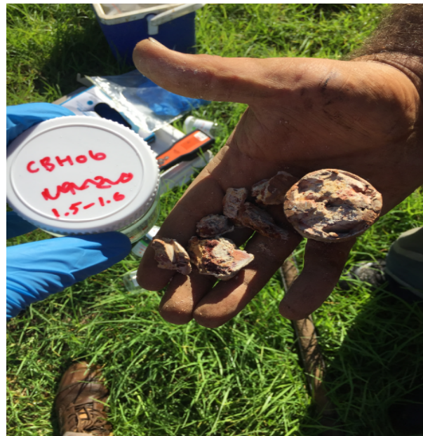
Photo 11: Sandstone encountered at CBH06
